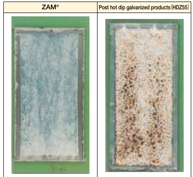
Appearances after 450 hours of sulfur dioxide test
