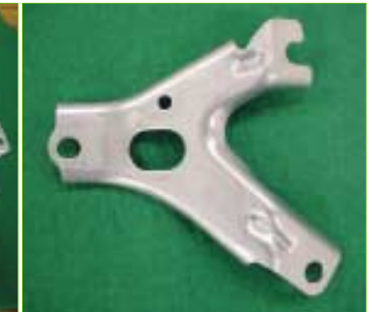
Surge tank stay
