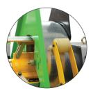
Heavy duty 5T decoiler with pneumatic snubber arm for improved safety.
