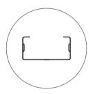
Web width range from 3½" - 12", up to 4+ profile sizes. Gauge range from 20 - 14 gauge (30 - 68mils).
