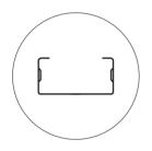
Web width range from 3½" - 6" with dual profile. Gauge range from 18 to 12 gauge (47 - 97mils)
