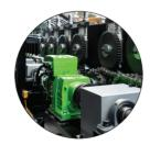
An automated servo driven raft to quickly and easily change web width, flange height and automatically adjust the tooling to match the new profile.
