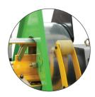
Heavy duty 3T decoiler with pneumatic snubber arm for improved safety.
