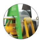
Heavy duty 3T decoiler with pneumatic snubber arm for improve safety.
