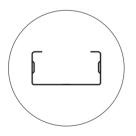
Web width range from 31/2" - 12", up to 4+ profile sizes. Gauge range from 18 - 12 gauge (43 - 97mils).
