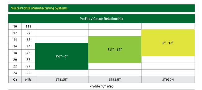
Multi-profile systems are built with multiple specified profiles. Customers can select from the range shown above.
