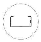
Web width range from 2½" - 6", up to 4+ profile sizes. Gauge range from 22 - 16 gauge (17 - 54mils).
