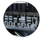
Unrivalled versatility with 12 punching functions that allows walls, truss and floors to be constructed using a single steel profile.
