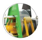
Heavy duty 5T decoiler with pneumatic snubber arm for improved safety.
