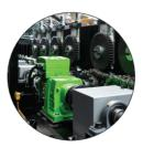
An automated servo driven raft to quickly and easily change web width, flange height and automatically adjust the tooling to match the new profile.
